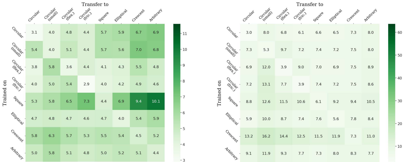
Fig. 12. Cross transfer pose estimation accuracy between the tested objects when including the initial grasp pose in the state (feature combination 9). Transfer scores include (left) position RMSE in mm and (right) orientation errors in degrees .
