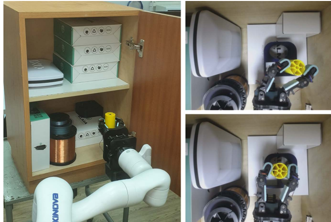
Fig. 1. Manipulating an object within an occluded cabinet using a robotic arm and an underactuated hand into a target slot. Visual perception is not available within the cabinet and, therefore, the hand must use haptic perception. We assume that the position of the hole relative to the robot is known.
