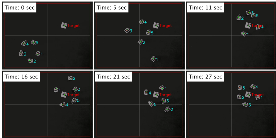
Fig. 16: A set of five MGR agents reaching a target using a trained policy while maintaining distance among them. The policy was trained on a simulation based on CR-Net-S.
