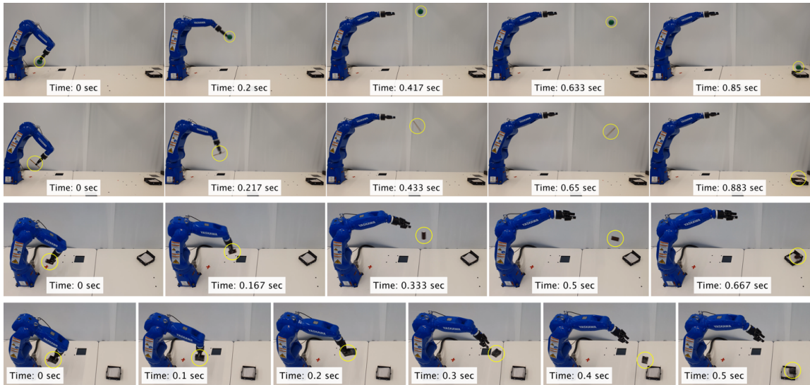
Figure 5.7: Snapshots of four throws (from top to bottom): squeeze ball ( d_g = 180\text{cm} ), pencil ( d_g = 180\text{cm} ), cylinder ( d_g = 140\text{cm} ) and box ( d_g = 90\text{cm} ). Objects are marked with a yellow circle for better visualization.
