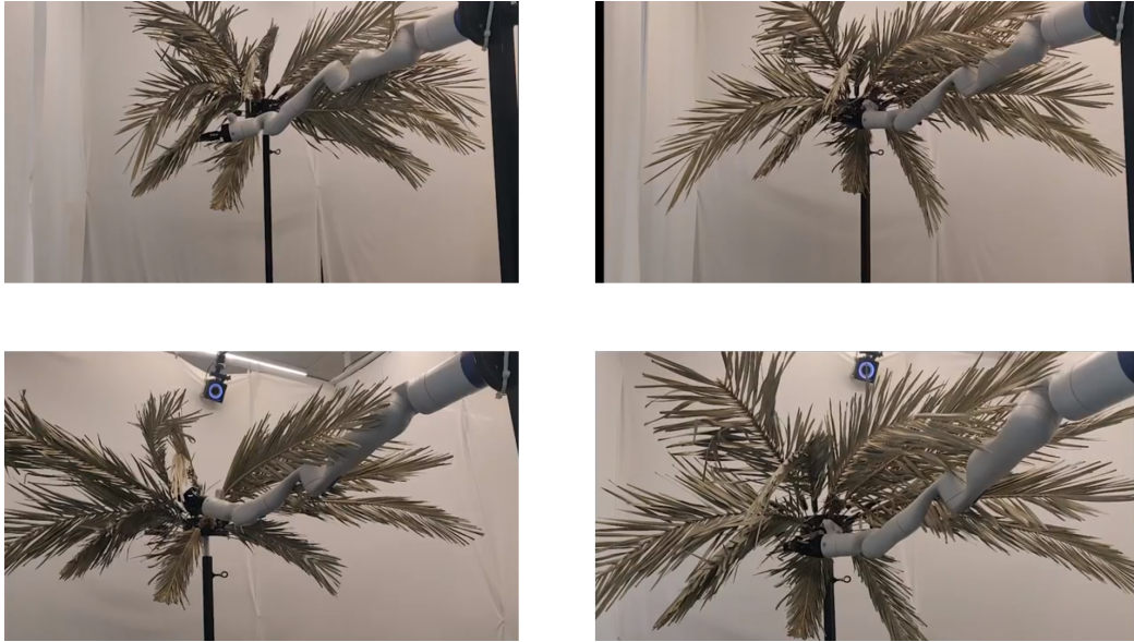
Figure 5.31: Kinova gen3 roll-outs of the optimal path for scenario III with a tree mock-up on different approach points.
