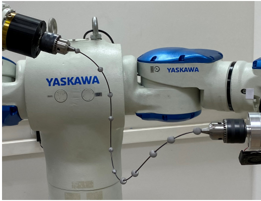
Figure 4.4: Shape estimation of a wire configuration using only F/T measurement. The circular blue markers are the ground-truth measured using a motion capture system and the solid curve is the estimation. Average shape estimation error along the wire is 5.81 mm.
