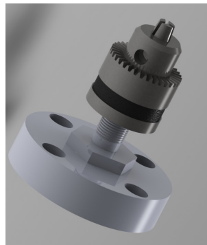
Figure 3.1: A chuck gripper has been added to each arm, allowing it to hold a circular rod without slippage.
