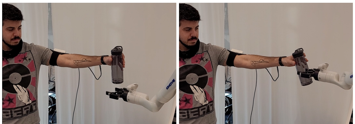
Figure 4.13: An HRC demonstration in which participant 1 hands-over a bottle to the robot.
